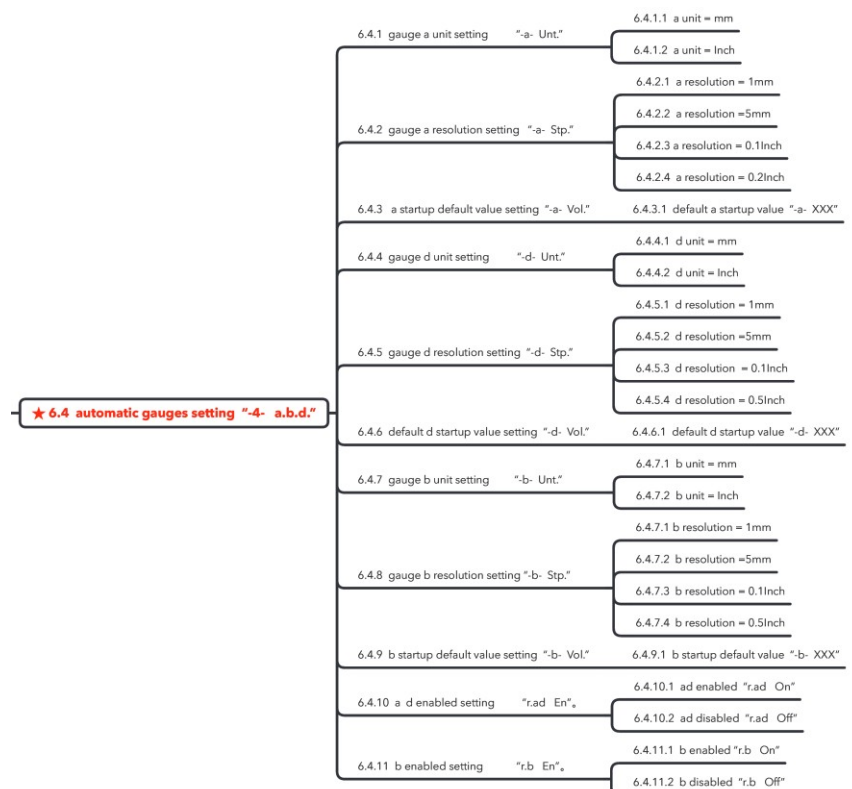
Fig.64 automatic gauge setting
